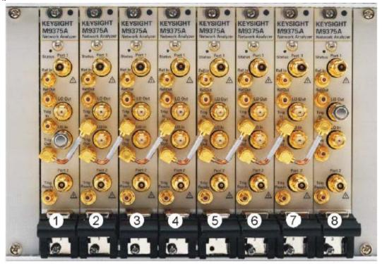
3. Install a semi-rigid cable (M9370-20006), seen in below figure, between the LO Out port and the LO In port on each of the module pairs (1 & 2, 2 & 3, 3 & 4, 4 & 5, 5 & 6, 6 & 7, and 7 & 8), hand tightening the connectors.
